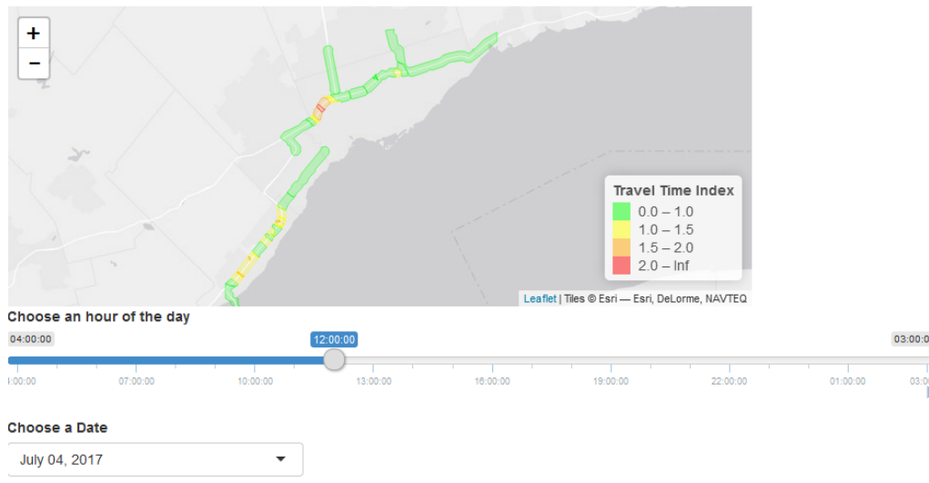
Figure 18: Screenshot of second panel showing ArcGIS-generated visualization of spatially interpolated hourly TTI averages
